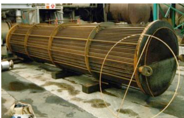
Figure 4: later Tasman Whessoe heat exchanger tube bundle (courtesy Joe Hotson)
