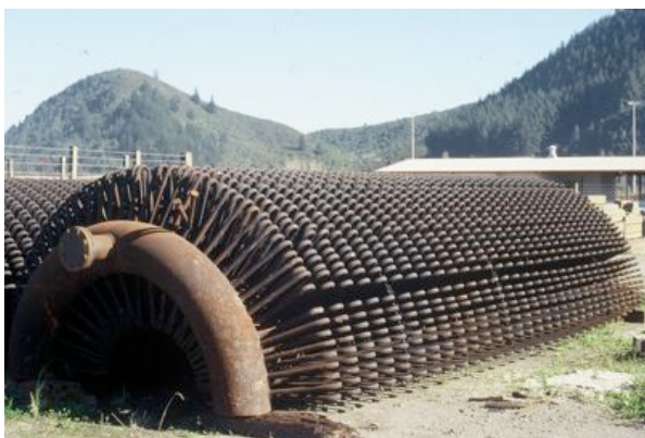
Figure 3: Original Tasman heat exchanger tube bundle (courtesy Joe Hotson)
