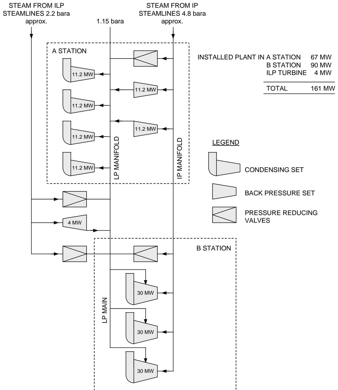
FIGURE 2.2 SIMPLIFIED STATION STEAMFLOW AND TURBINE ARRANGEMENT
